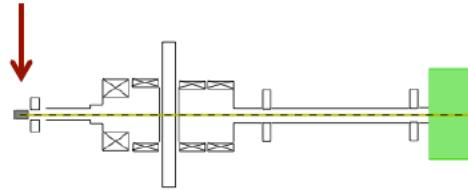
$22 \lambda_{\text{int}}$  Cu collimator (TAX) closed for dump-mode data taking
