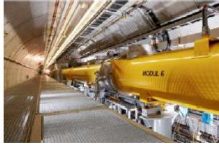
> TESLA type superconducting accelerating modules 1.3 GHz
