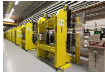
> FLASH2 variable gap undulators
