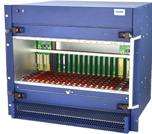
Schroff & ELMA 12 Slot MTCA.4 Chassis
