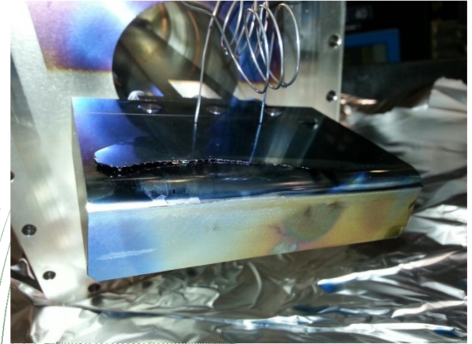
MEBT Chopper Target Rupture: FY2014
