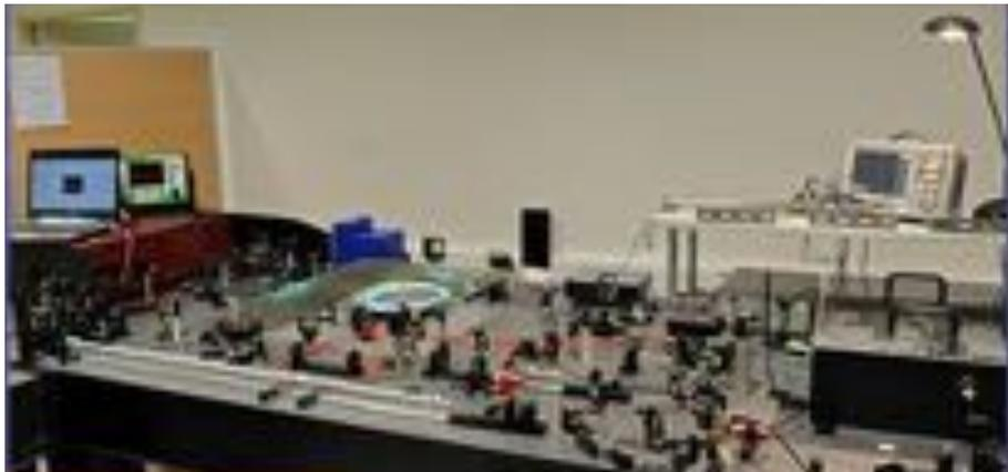
Table-top HHG source with a megahertz fibre laser: (25-40 eV) radiation; at 30 eV an average power of 143  $\mu\text{W}$  ( $3 \cdot 10^{13}$  photons/s).
