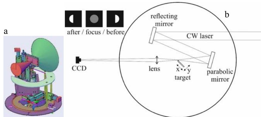
Experimental stand for study of the impact of 25 MeV laser-accelerated protons on biological objects. It is demonstrated the doses up to 10 Gy to the object can be transferred in a single shot. The technique of irradiating the cell culture HeLa Kyoto and measuring the fraction of survived cells is developed.
