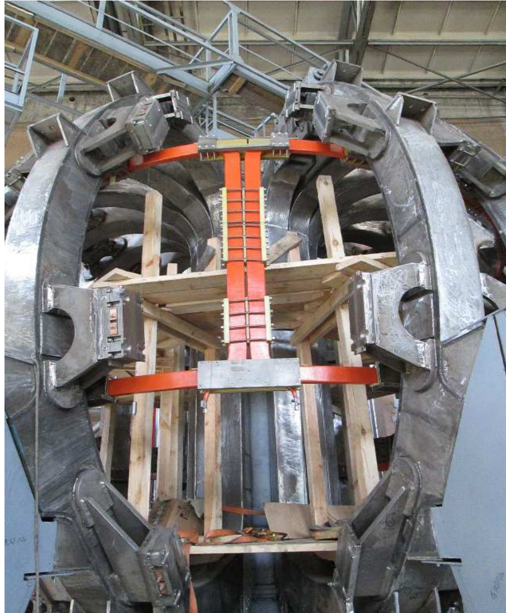
Placement of HF coils inside toroidal winding
