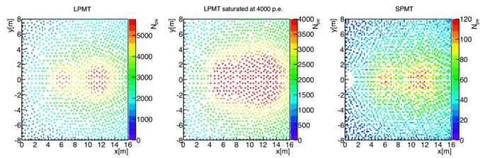
Example of double muon hit pattern seen by LPMTs without saturation, LPMTs saturated at 4000 p.e., and SPMTs
