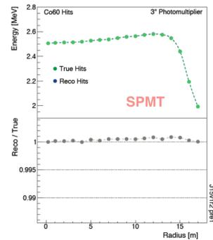
Simulated <sup>60</sup>Co calibration campaign at different radii. The reconstructed energy of LPMT with 5% assumed non-linearity is biased compared to MC, while the bias can be corrected by the SPMT measurement
