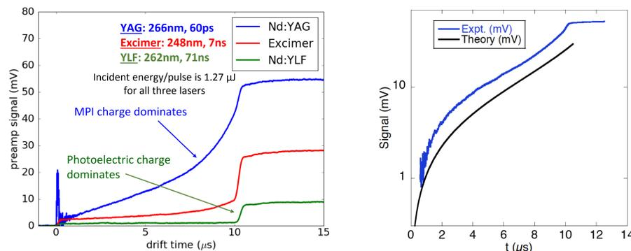
Calculated MPI signal using the CSU cross section reproduces the shape of the BNL/SBU data (blue curve) well and the absolute signal to within  $\sigma_2$  uncertainty.
