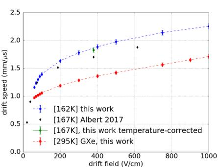
The drift speed increases with drift field.
