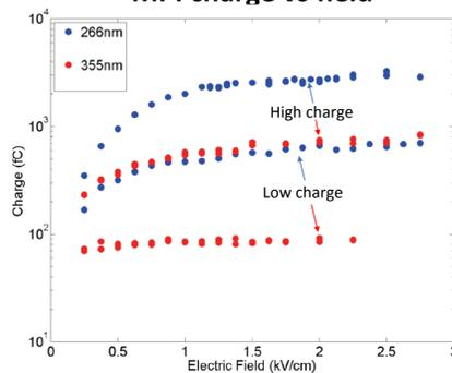
The collected charge is constant for electric fields higher than 1kV/cm, independent of the ionizing photon wavelength.
