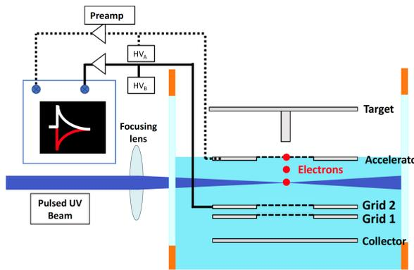
Laser focused between Accelerator and Grid 2.
