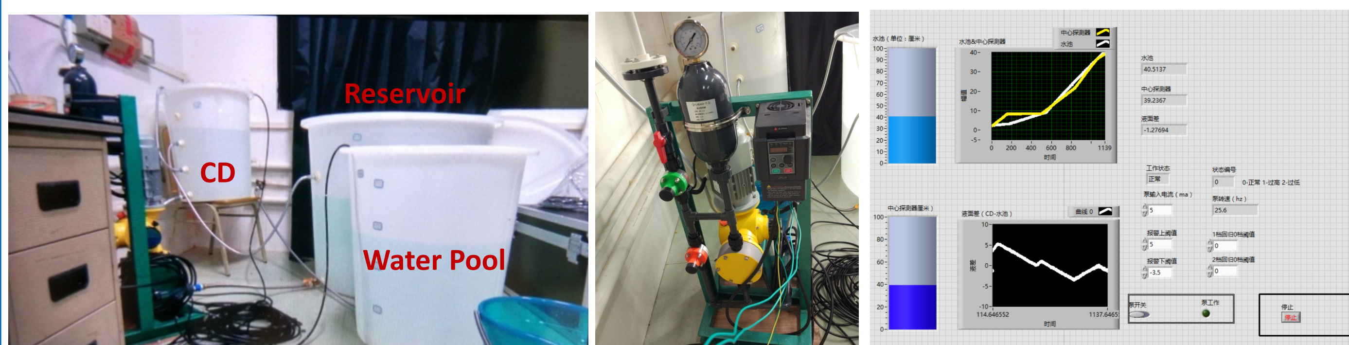
The test setup for the filling procedure of JUNO. CD, reservoir and water pool are represented by plastic vessels equipped with hydrostatic pressure sensors.
