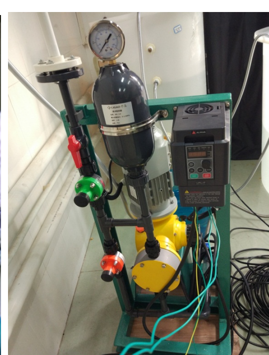
The electric pump used for circulating the water from vessel to vessel.
