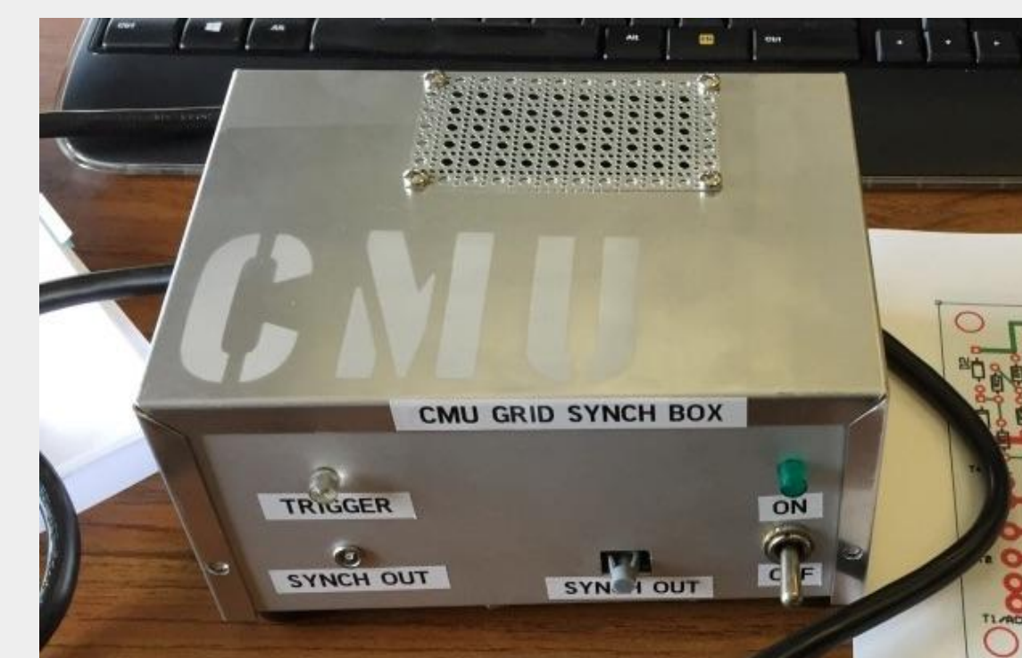
Grid synch box installed at the KATRIN detector system.
