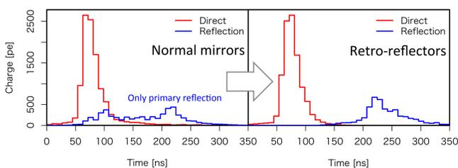
With retro-reflectors (right) the reflected light is well separated in time.
