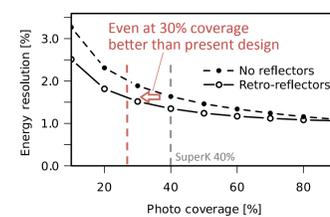
Energy resolution mostly depends on the number of collected photons. The more PMTs we have the less reflectors we can place, so the sensitivities converge.
