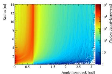
At each solid angle we measure not only the photon flux but also their direction distribution, which allows modeling of reflections including scattering effects.
