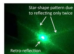
Laser beam pointed at a micro-prism tape reveals different types of reflections. ↑
