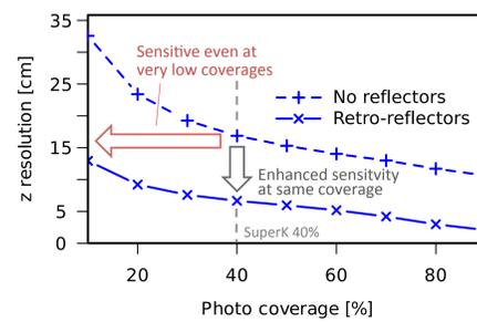
The enhanced position and angle sensitivities due to parallax result from a new information class (photon direction) and are thus effective for a wide range of coverages.
