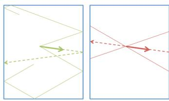
↑ Reflected light path for normal mirrors (left) and retro-reflectors (right).
