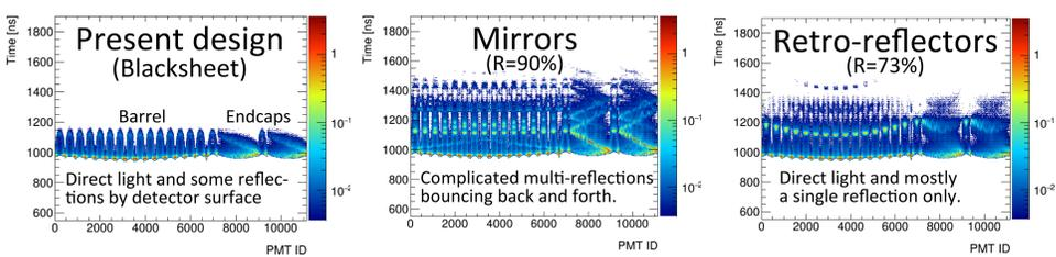
Simulation using Geant4<sup>1</sup>-based WCSim<sup>2</sup>. Blacksheets between PMTs are replaced with reflective materials. The complicated multi-reflection time signatures due to mirrors disappear almost completely with retro-reflectors. (side-going electron in SuperK<sup>3</sup> sized detector)
