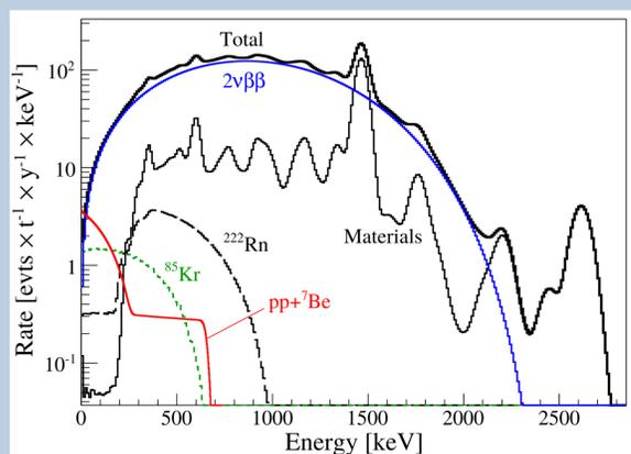
Predicted background spectrum from detector materials and internal contamination.
