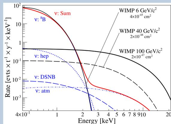
Nuclear recoil spectrum for CNNS from  $\nu_{\odot}$ , diffuse supernova background and  $\nu_{atm}$ .
