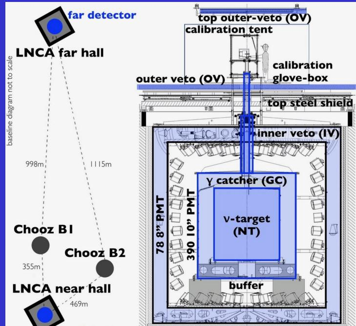
The Double Chooz experiment goal is the precise measurement of the  $\theta_{13}$ neutrino mixing angle. It measures  $\bar{v}_e$  -flux from the two nuclear reactors of the Chooz NPP with total thermal power ~8.4 GW using two identical detectors. The near (ND) and far (FD) detectors are respectively at ~400 m and ~1050 m.
