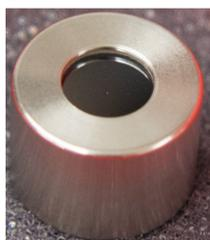
Figure 3. PIPS Canberra detector.
