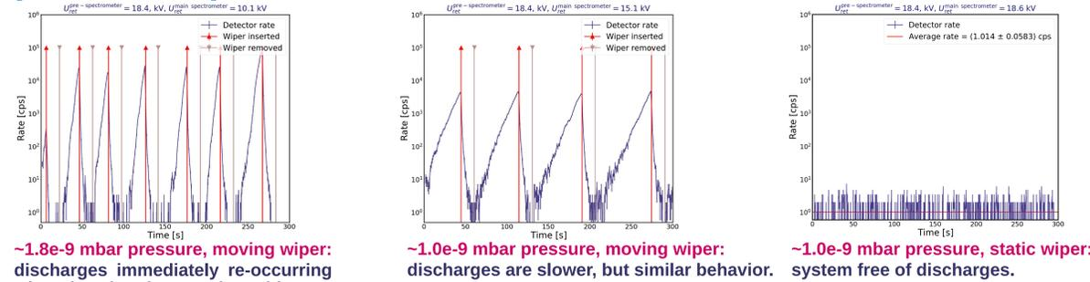
~1.8e-9 mbar pressure, moving wiper: discharges immediately re-occurring when the wiper is moved outside.
