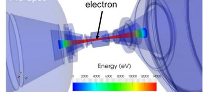
Simulation of an electron trapped inside the interspectrometer Penning trap (from L. Kippenbrock).
