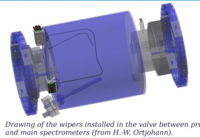
Drawing of the wipers installed in the valve between pre- and main spectrometers (from H.-W. Ortjohann).
