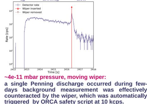
~4e-11 mbar pressure, moving wiper: a single Penning discharge occurred during few-days background measurement was effectively counteracted by the wiper, which was automatically triggered by ORCA safety script at 10 kcps.
