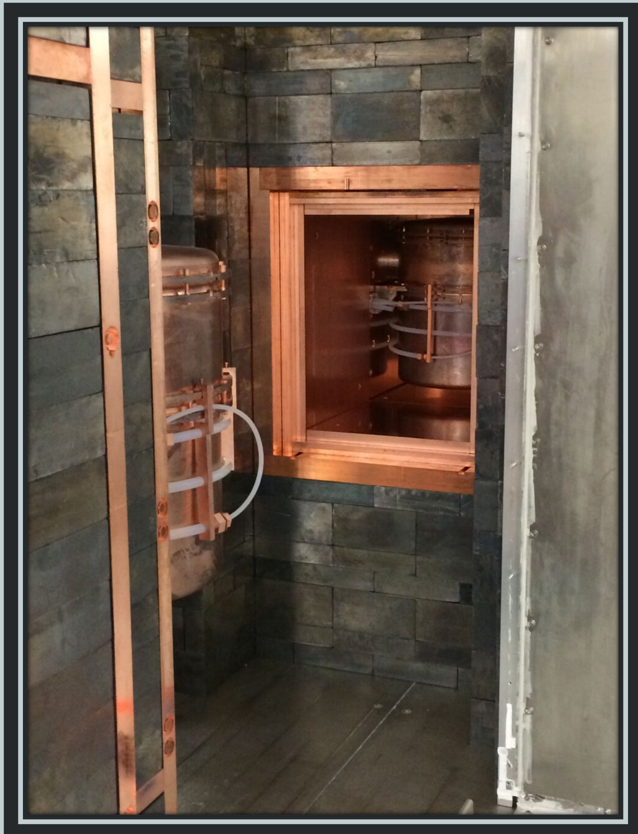
Figure 2: View of Module 1 in the compact lead and copper shielding (background), with Module 2 waiting to be inserted into the shield (foreground).
