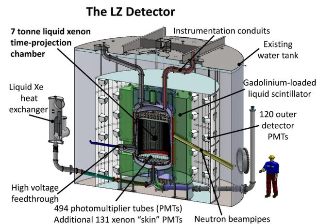
**Figure 2:** The LZ experiment, consisting of the LXe-TPC, viewed by top and bottom PMT arrays, plus a LXe "skin" and Outer Detector (OD) to veto gammas and neutrons.
