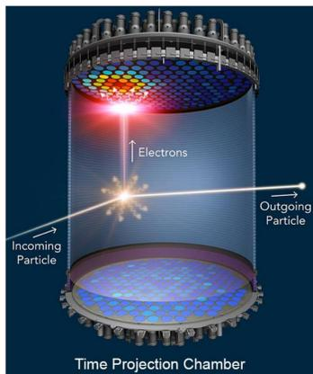
**Figure 1:** LXe-TPC operation principle. A particle interacting in the LXe produces a prompt scintillation signal (S1) and ionised Xe atoms. The released electrons are swept upwards by an electric field and extracted into the gas phase to produce electroluminescence (S2). These two signals are used to reconstruct both event energy and position.
