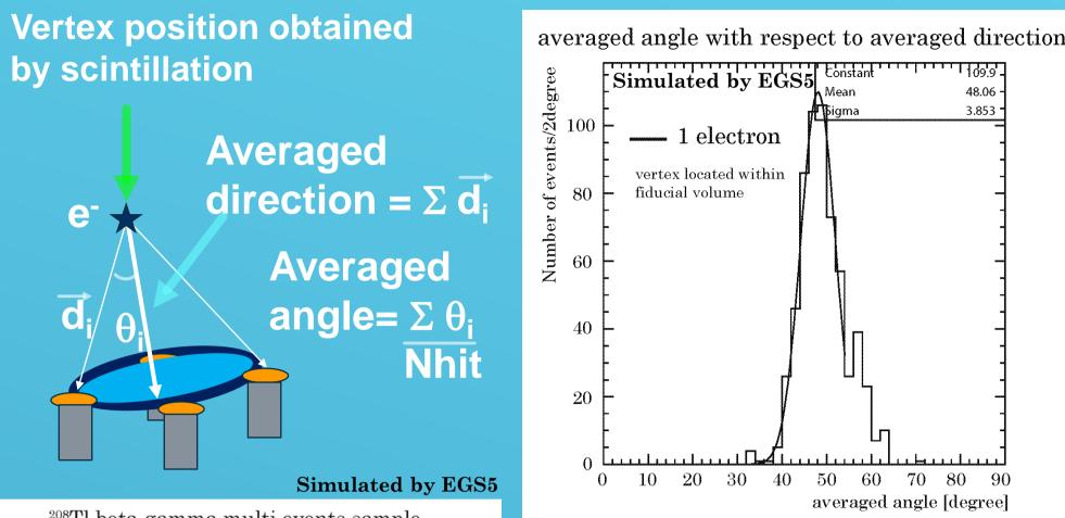
The averaged angle distribution with respect to the averaged direction of single electron has a peak at ~48 degree which is almost same value as Cherenkov angle in Anisole.
