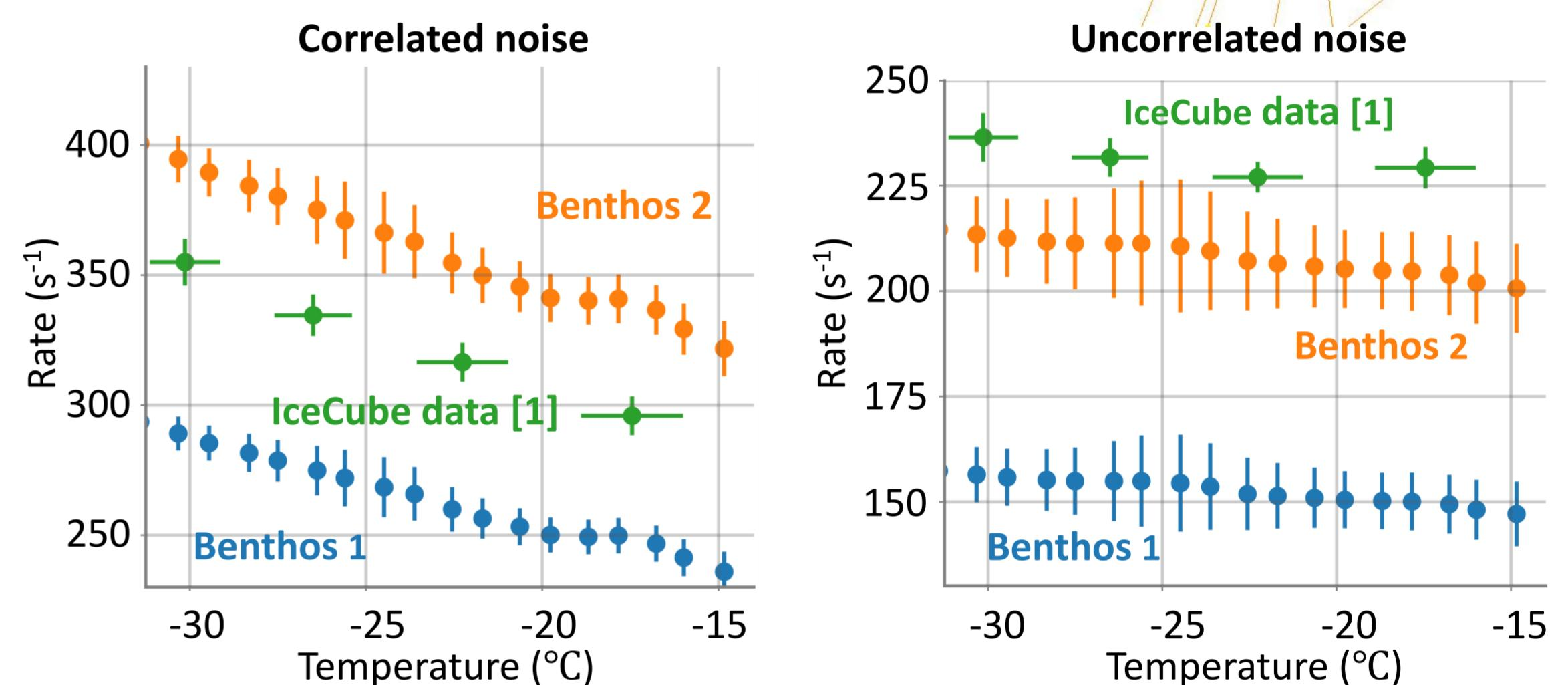
Simulated temperature dependence in good agreement with experimental data. Decreases with temperature due to change in yield.
