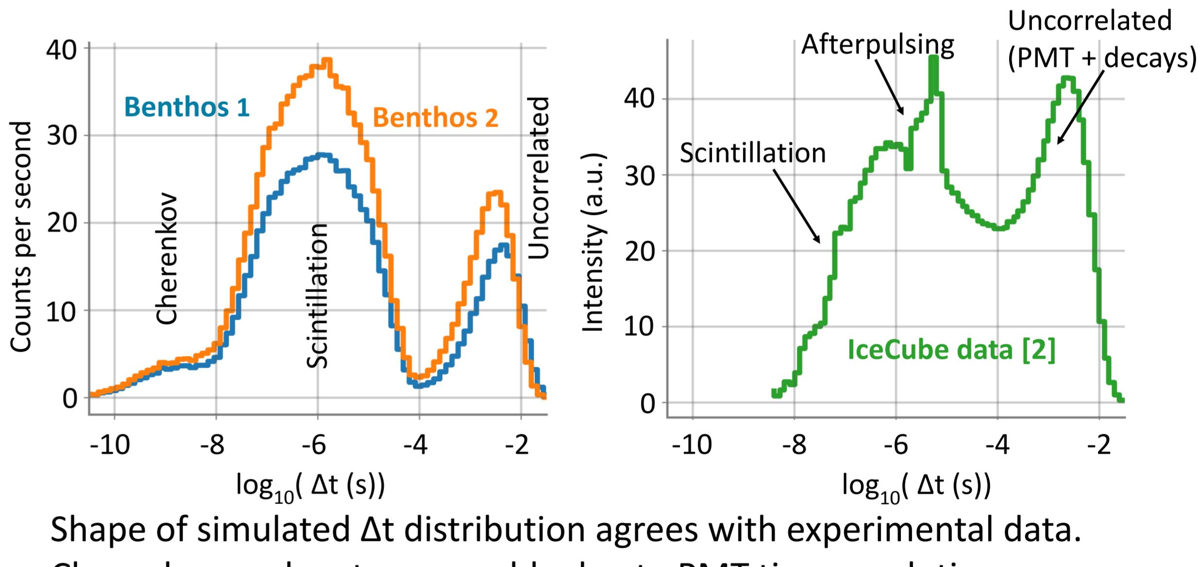
Shape of simulated  $\Delta t$  distribution agrees with experimental data. Cherenkov peak not measurable due to PMT time resolution.
