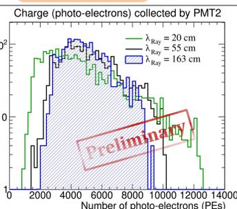
Attenuation due to the cathode and the ground grid in ProtoDUNE-DP
