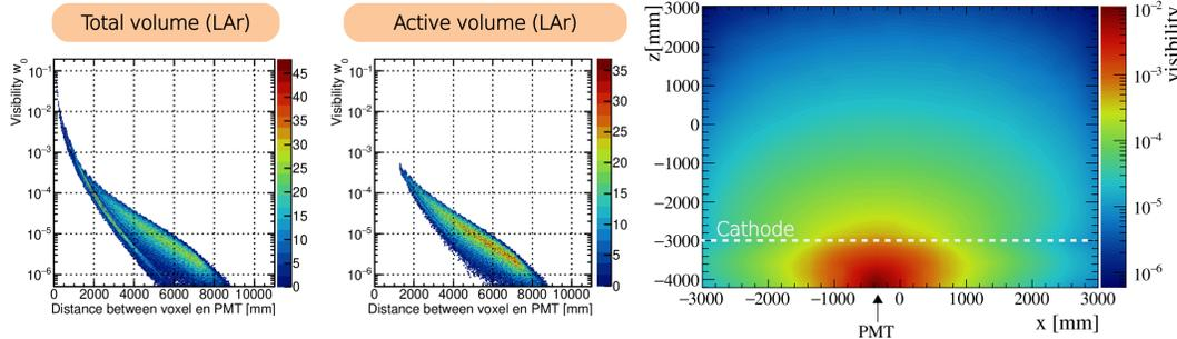
For DUNE, investigation of the possibility to parametrise the visibility as a function of the voxel-PMT distance
