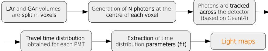
Light maps were produced using LightSim software, for ProtoDUNE-DP and 3x1x1 demonstrator
