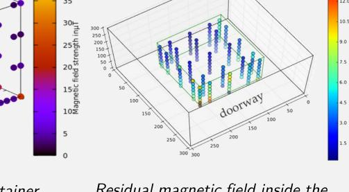
Residual magnetic field inside the container, ~ 5 µT. Weak spots are strengthened with additional FINEMED layers around boxes
