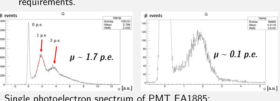
Single photoelectron spectrum of PMT EA1885: Measurements performed at different light (LED) intensities.
