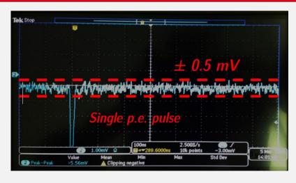
Low noise levels of  $\pm 0.5 \,\mathrm{mV}$ , Noise-to-Signal-ratio of ~ 7 %
