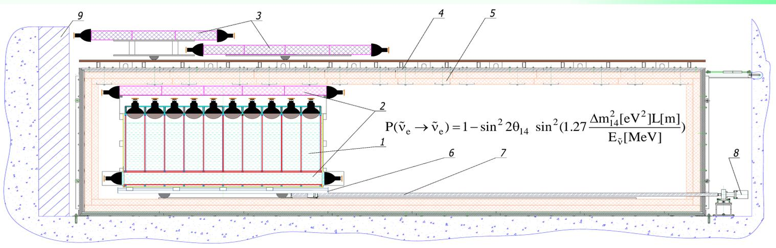
Location in building and general scheme of experimental setup. 1 – detector of reactor antineutrino with 50 PMT-9354, 2 – internal active shielding, 3 – external active shielding (umbrella), 4 – steel and lead passive shielding, 5 – borated polyethylene passive shielding, 6 – moveable platform, 7 – feed screw, 8 – step motor, 9 – iron shot.
