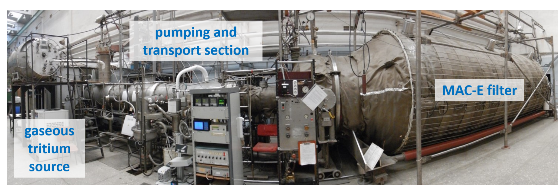
▲ The Troitsk \nu -mass experiment is a technological predecessor of KATRIN. A TRISTAN 1-mm prototype detector was installed into the spectrometer to measure electrons from different sources.
