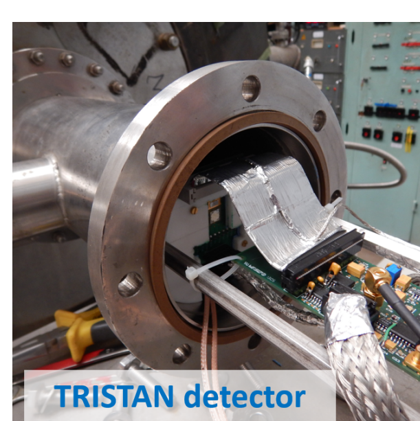
▲ The Troitsk \nu -mass experiment is a technological predecessor of KATRIN. A TRISTAN 1-mm prototype detector was installed into the spectrometer to measure electrons from different sources.
