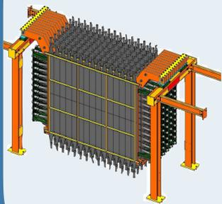
The Muon Range Detector (MRD) was inherited from the SciBooNE experiment and is being fully refurbished by the ANNIE Collaboration. It consists of alternating layers of plastic scintillator and steel plates. The scintillator layers are segmented strips and alternate between horizontal and vertical orientation to allow for x-y tracking of particles passing through multiple layers.
