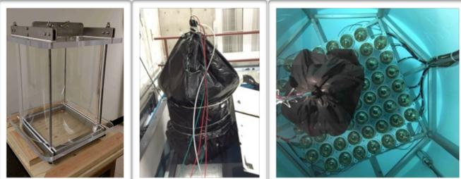
The NCV was filled with 95 liters of Eljen EJ-335 (0.25%) Gadolinium doped liquid scintillator. Two waterproofed PMTs were optically coupled to the top of the acrylic vessel. To optically isolate the NCV from the water volume while running in "Hefty mode", it was wrapped in commercially available polyethylene liners.
