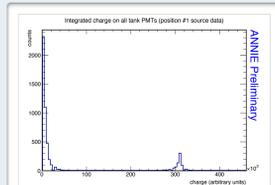
In Phase I, the 60 upward-pointing PMTs (shown being installed on the left) act as an active veto for charged-current neutrino interactions in the water volume and to cosmic-ray muons entering from above. The plot on the right shows a charge cut used to remove random cosmic-ray muons from our source calibration sample.
