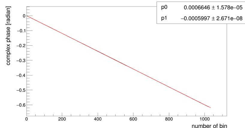
Time extraction based on straight line fit
