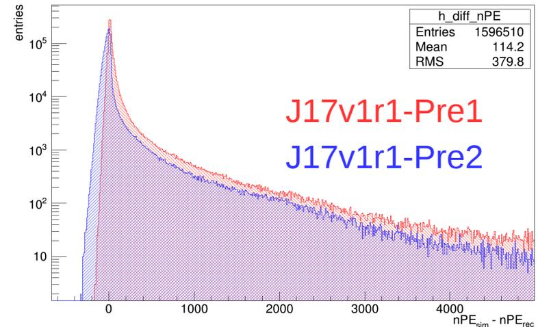
*Comparison of charge reconstruction from last validation cycle and before*
