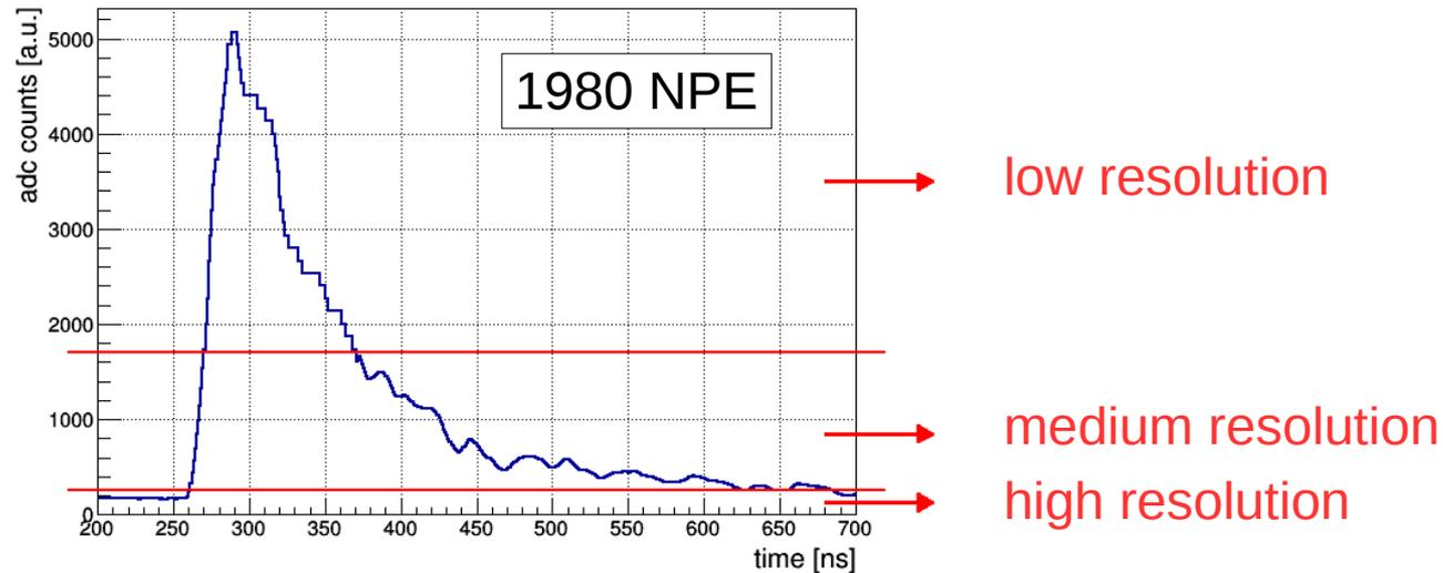
*Waveform example of center muon event*
