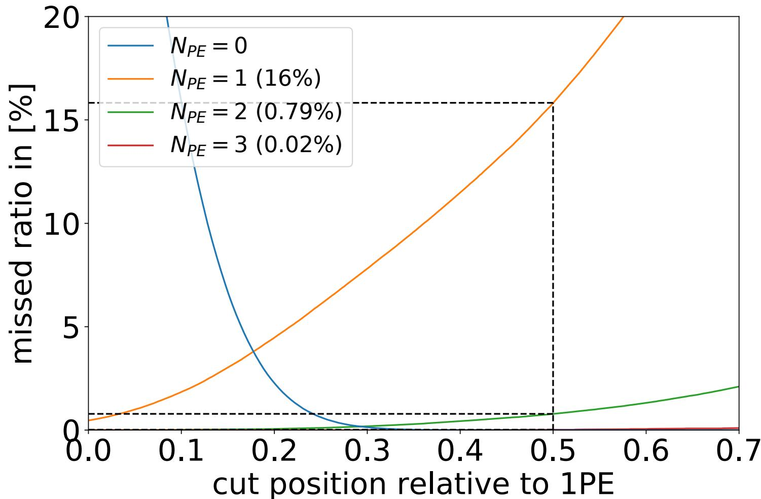
Trigger efficiency <16% for 0.5 PE trigger level
