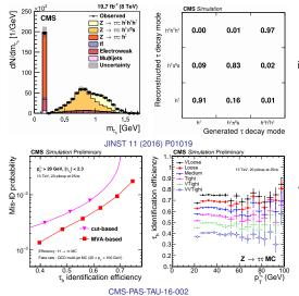
$$\label{eq:theta} \begin{split} \tau_h \mbox{ reconstruction in decay modes, as} \\ introduced \mbox{ for Run I. Decay modes are} \\ reconstructed \mbox{ correctly at 83 \% or} \\ higher \end{split}$$
