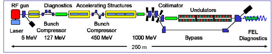
The ~1 GeV linac of the SASE VUV laser provides a unique test facility for both the XFEL and ILC. Currently constructed
