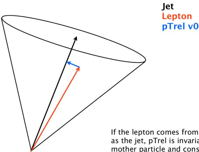
If the lepton comes from the same mother particle as the jet,  $pT_{rel}$  is invariant under the boost of the mother particle and constrained by its mass.
