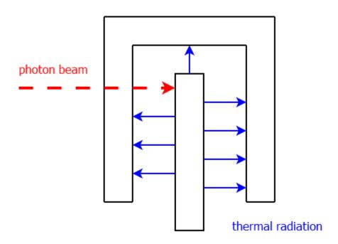
$$P \sim \sigma \varepsilon A \left( T_{t \operatorname{arg} et}^4 - T_{cooler}^4 \right)$$
