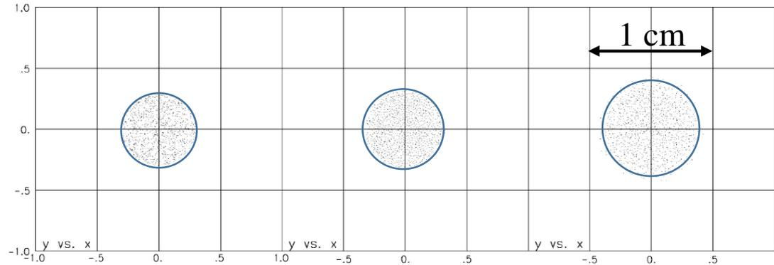
Fig. 4-11 Beam size (cm) at gun exit. ( $I = 0 / 100 / 600$  mA,  $E_k = 2.3$  MeV)
