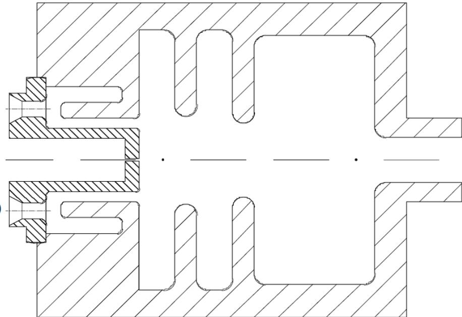
Cross Section: overall length 100 mm, maximum inner radius  $\approx 40$  mm
