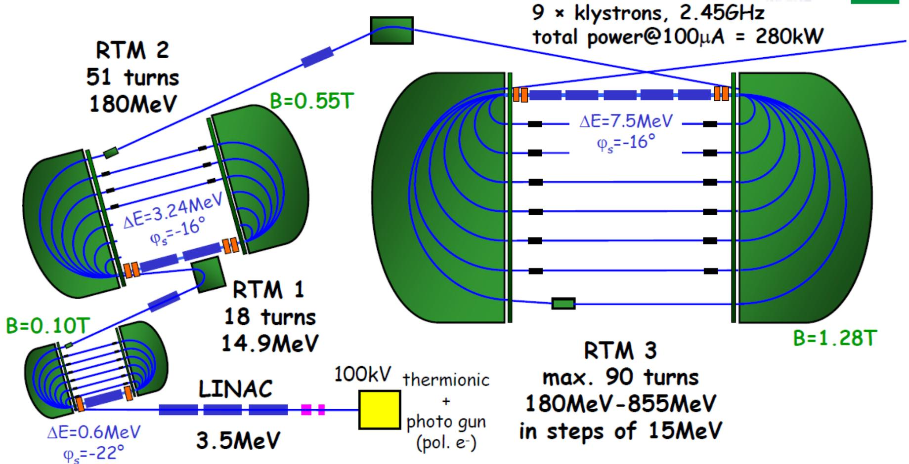
beam parameters: 100μA max cw current (86kW beam power)
