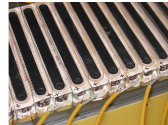
Short period SC wigglers ( B_0 = 2-2.2 Tesla, \lambda_0 \sim 30-34 mm)
