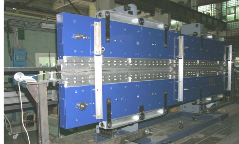
Undulator (prototype) for XFEL (Germany, 2014)
