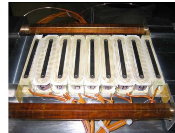
Medium period SC wigglers ( B_0 = 3.5-4.2 Tesla, \lambda_0 \sim 48-60 mm)
