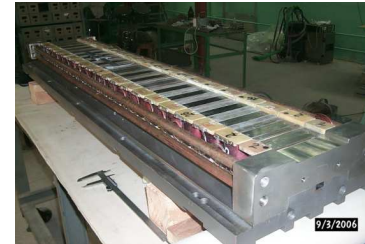
Long period SC multipole wigglers ( B_0 = 7-7.5 Tesla, \lambda_0 \sim 150-200 mm)
