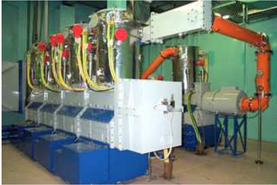
Four modules RF generator for microtone in the NovoFEL for 8 cavities
