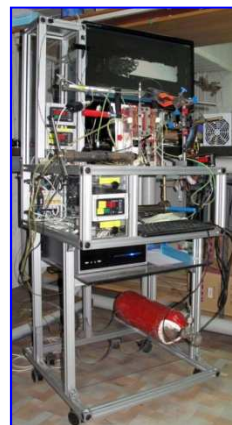
Universal mini laboratory for the physical and chemical process study in supercritical fluids.
