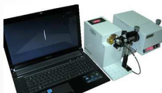
Spectroscopic refractometer for the refractive index measurements of liquids and solids.
