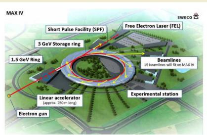
MAX-IV: first source with top-up linac injection (also used for SPF)
