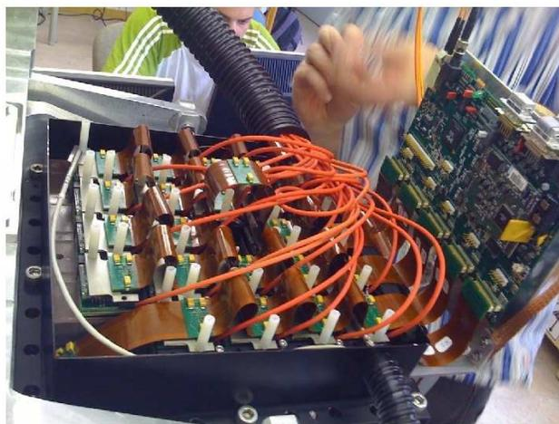
Fig. 5: Front-end electronics: Kapton cables each connected to 5 PMFs sitting on top of the MAPMTs.
