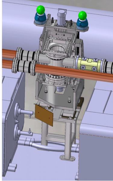
Fig. 1: Schematic drawing of the ALFA Roman Pot station.
