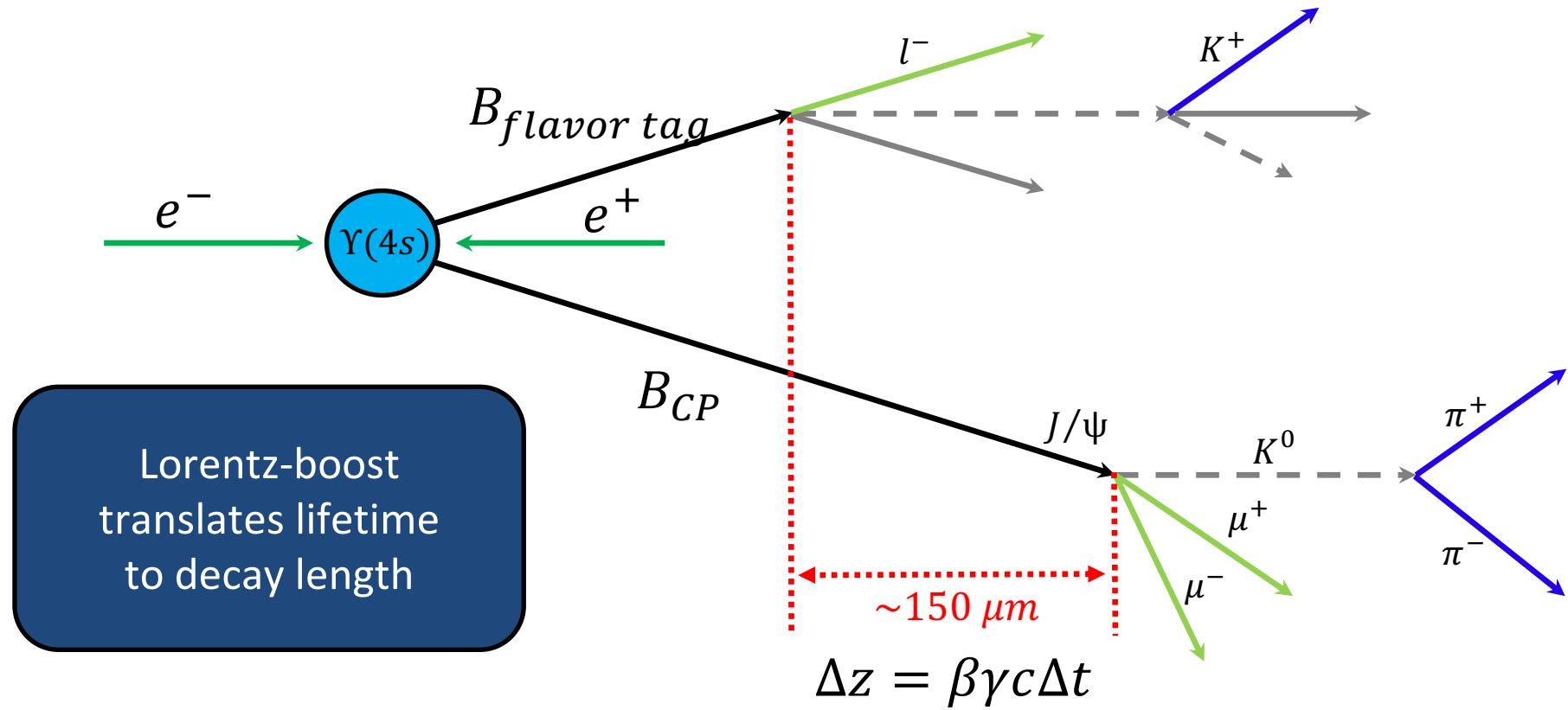
Precise vertexing → High resolution and light inner detector
