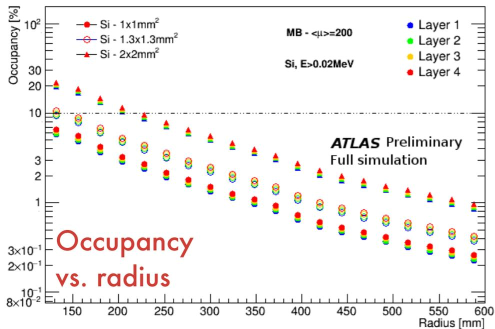
Granularity of  $1.3 \times 1.3$  mm<sup>2</sup> keeps occupancy  $< 10\%$  at all radii
