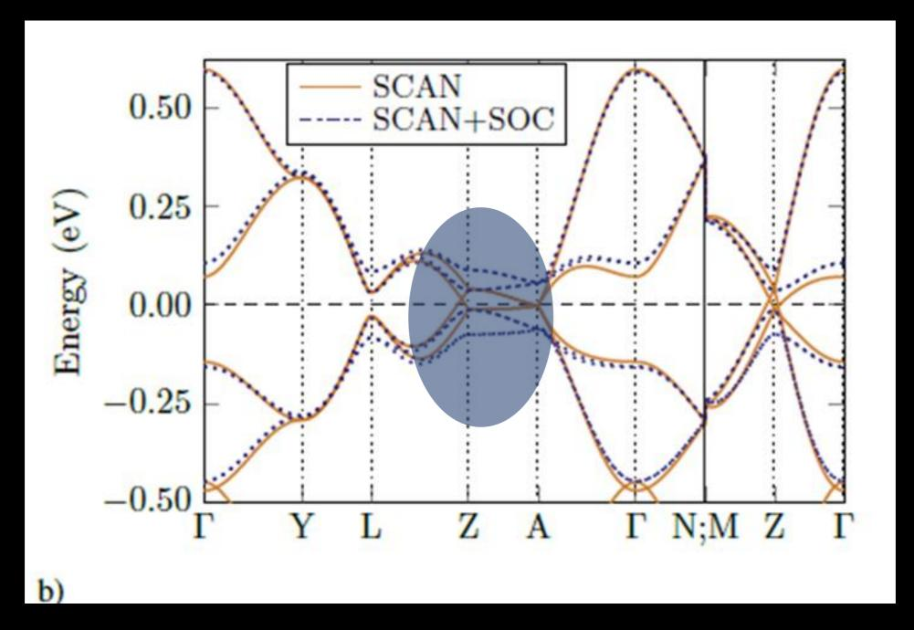
Linear crossing gapped out by spin-orbit coupling Band gap ~ 50 meV, much smaller gaps should be possible
