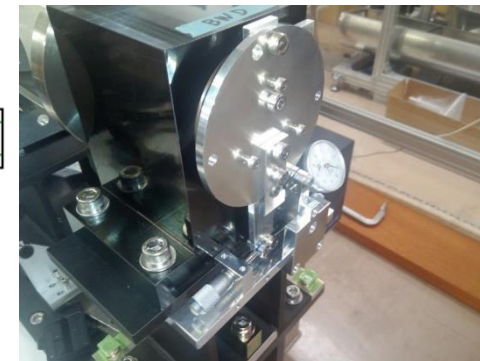
Angle fine control jig for PXD mount
