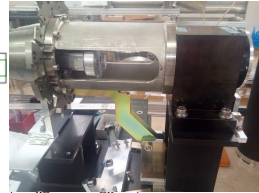
Support arm to control mechanical sagging
