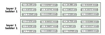
Results of alignment procedure using mixture of cosmic and collision data. The worst results are for *u* alignment parameters.
