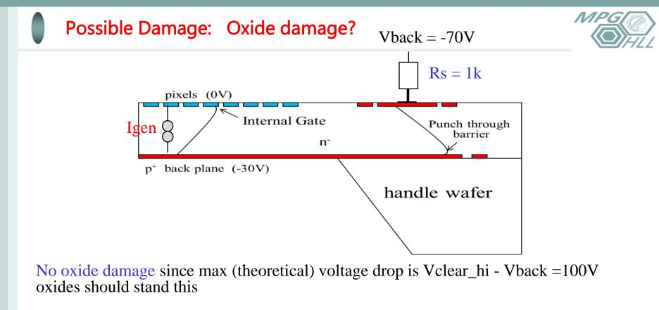
Even relaxed: max voltage drop cannot occur in the matrix, for instance: Igen =  $70mA \rightarrow all$  the voltage drops over Rs In addition: Rs >> Ron (Clears) all in parallel, matrix will be kept at frontside potentials
