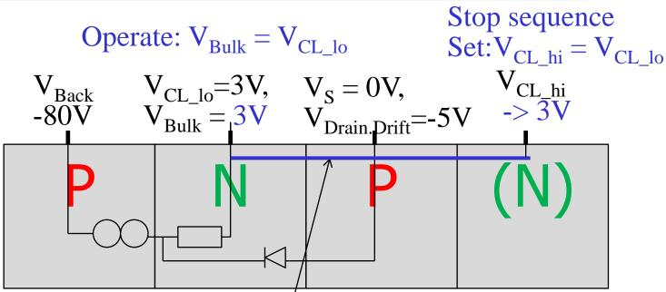
Thyristor becomes a pnp bipolar transistor with partially ,floating' gate. Part of the generated electrons will be amplified other part extracted N - contacts.
