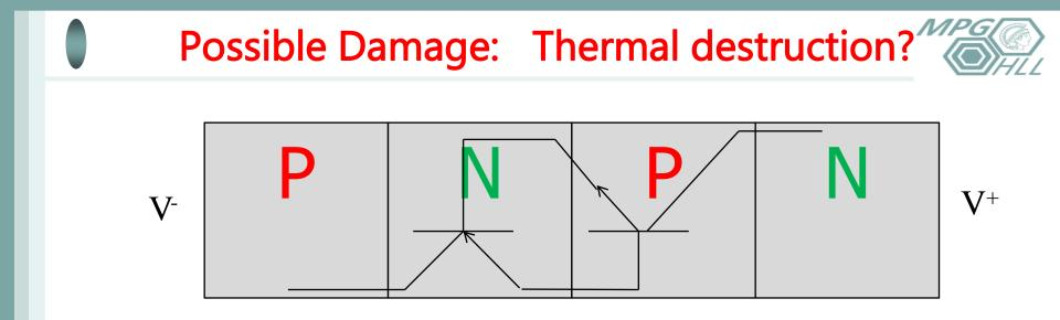
Forward bias of base emitter diodes The by intention -> thyristor ov parasitically -> latch up as in CMOS chips get destructive (thermal) and non destructive latch up possible device switchs off if voltage drops and current falls below holding current
