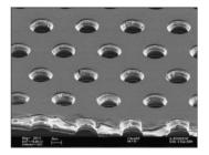
Electron microscope picture of a section of typical GEM electrode, 50  $\mu m$  thickness.\*
