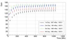
Long time measurements **before corrections** for 4 consecutive days with ceramic GEM at 740 V. Long time measurements after corrections at 740 V, 1 atm and 299.5 K.
