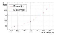
$V_{GEM}$  vs. gain for ceramic GEM
