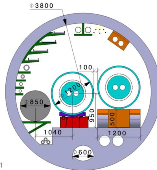
If HE-LHC can work in 3.8m Ø ... it will feed-back to FCC tunnel design!
