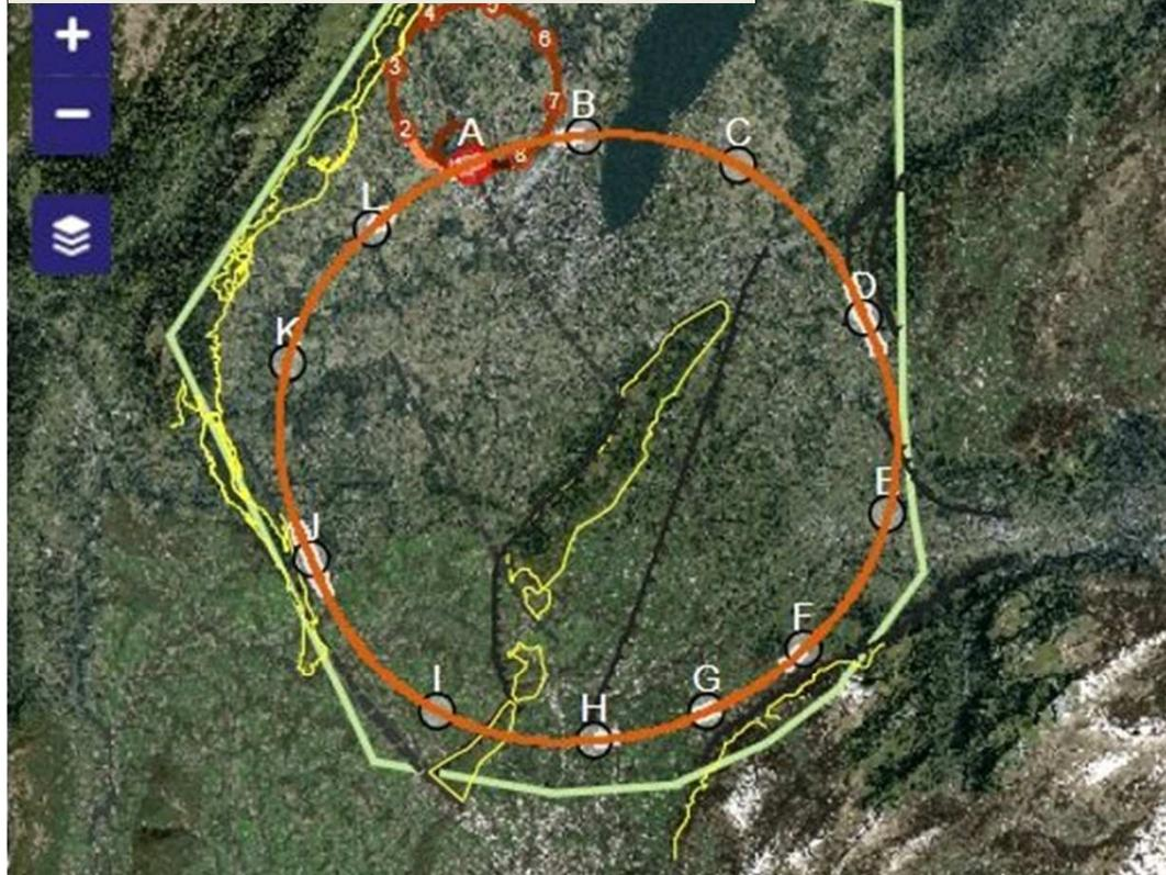
Optimisation in view of accessibility surface points, tunneling rock type, shaft depth, etc.
