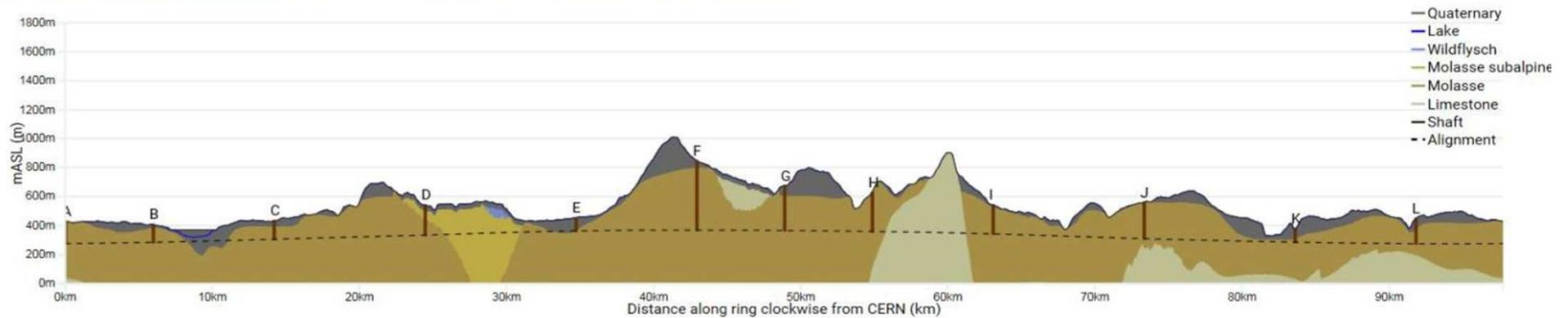
Geology Intersected by Tunnel      Geology Intersected by Section
