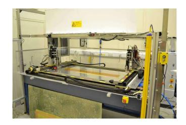
Test signal transmission through bustape at different stages of petal production → Get robotic tape tester
