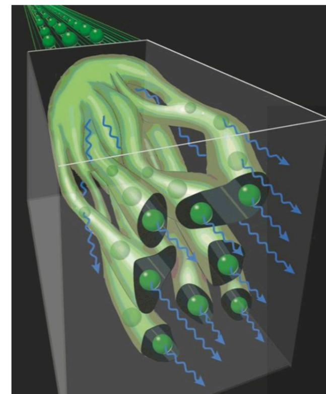
Current filamentation instability is observed and studied in a laboratory environment with a 60 MeV electron beam and a plasma capillary discharge. Multiple filaments are observed and imaged transversely at the plasma exit with optical transition radiation.
