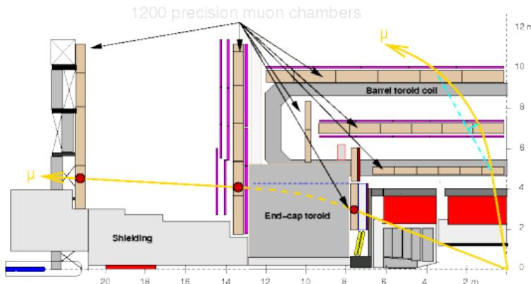
Air core toroid magnet to minimize multiple scattering:
