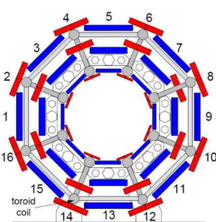
**Large (blue color) and Small (red color) sectors of the Barrel part of Muon Spectrometer**
