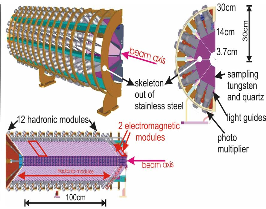
> Cherenkov quartz-tungsten sampling calorimeter for CMS@LHC with quartz plates as active medium and tungsten as absorber → compact, radiation hard and fast
