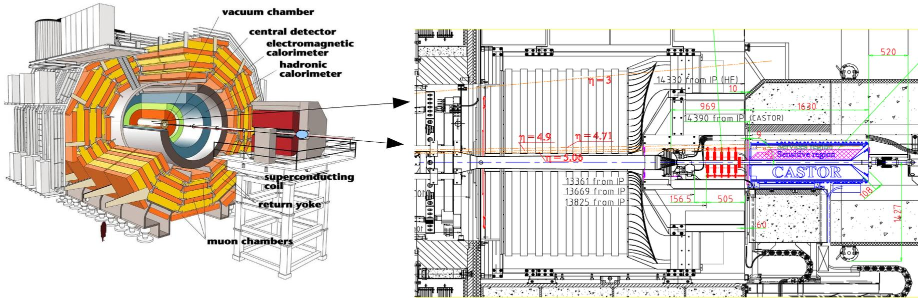
> Forward calorimeter ( $-6.6 < \eta < -5.2$ ) for low-x parton dynamics, minimum bias event structure, diffraction, cosmic ray related physics in low-luminosity proton-proton and heavy-ion collisions
