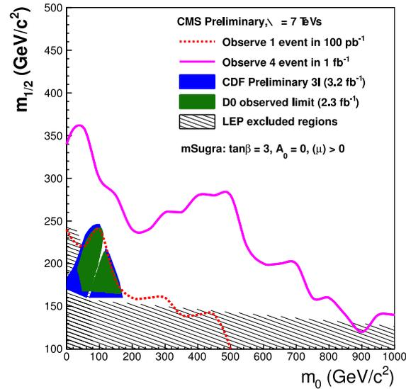
Figure 4: Estimated 95% C.L. exclusion limits for the like-sign dilepton SUSY search, expressed in mSUGRA parameter space. The expected background from the standard model at  $100 \text{ pb}^{-1}$  ( $1 \text{ fb}^{-1}$ ) is 0.4 (4.0) events; we have assumed an observed yield of 1 event (4 events) for the purpose of setting these exclusion limits.
