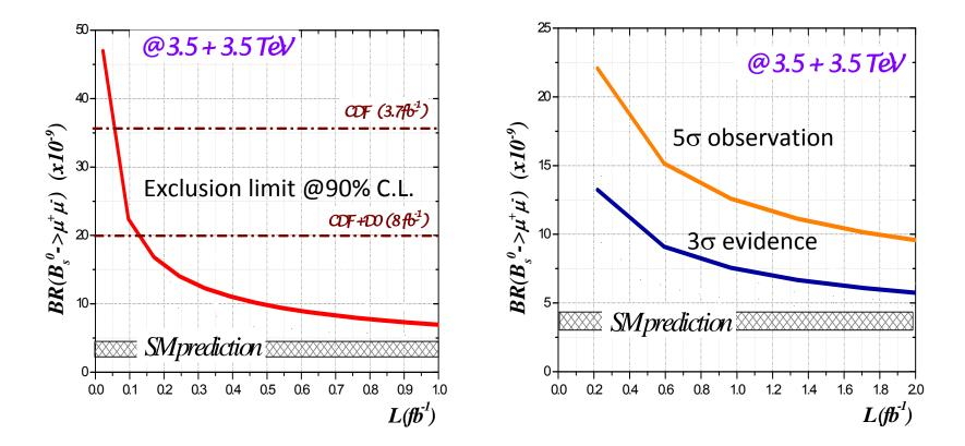
With 0.1fb<sup>-1</sup> we can improve the current best experimental limit With 1fb<sup>-1</sup> we can expect to exclude BR up to  $\sim$ 7x10<sup>-9</sup> @ 90% CL
