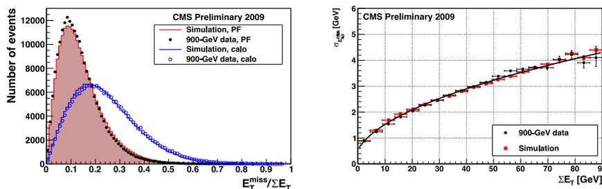
Figure 4: Left: distribution of the particle-based (solid) and calorimeter-based (hollow)  $E_T^{\text{miss}}/\Sigma E_T$  in the data (dots) and in the simulation (histogram). Right: resolution of the particle-based  $E_{x,y}^{\text{miss}}$  as a function of the particle-based in the data (dots) and in the simulation (squares).
