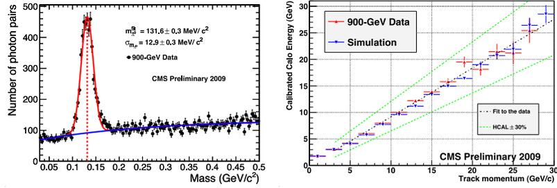
Figure 2: Left: photon-pair invariant-mass distribution in the barrel ( $|\eta| < 1.0$ ) for the data. Right: average calibrated calorimeter response as a function of the track momentum for the 900 GeV data (light upwards triangles) and for the simulation (dark downwards triangles). The dashed lines show the same quantity when the HCAL raw response is changed by  $\pm 30\%$
